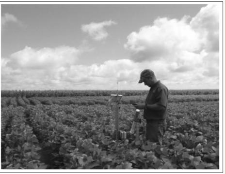
Fig. 1. A wireless system that monitors soil moisture and plant canopy temperature is being installed.
